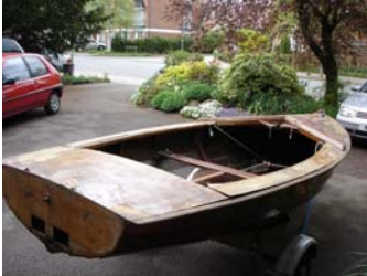
Decks about to fall off
